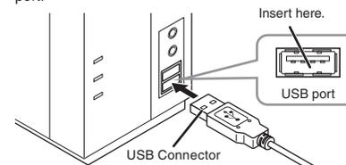
Carefully check the orientation of the connector and the place where you will connect the USB connector.
