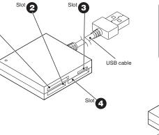
The LED of this product will flash when writing to or reading a memory card O not remove a memory card from the slot while the PC is writing to or reading from it Do not disconnect this product from the PC while it is writing to or reading from a memory card. Doing so may cause product damage and result in file damage or loss.
