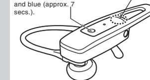
1 While this product is OFF, continue to press the multi-function button for approx. 7 seconds. The lamp will alternately blink red and blue.
