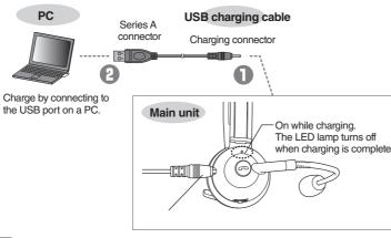
Connect the charging connector for the included USB charging cable to the charging connector on the product.
