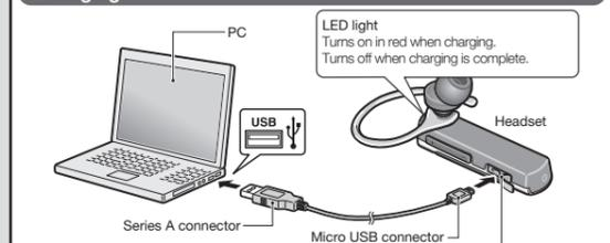
**When the battery charge is insufficient**
