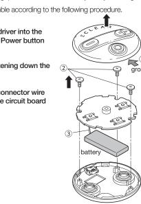
Be careful not to short-circuit the (+) and (-) terminals of the battery following removal, and fix tape over the terminals to insulate them.
