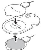
(3) Wind electrode cords of gel pads onto the protective plate.
