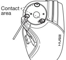
Take care not to damage the optical sensor when cleaning the area.
