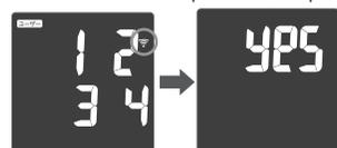
When the connection is completed, the wireless communication display on the display section of the body composition indicator changes from blinking to lit.
