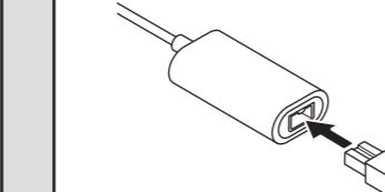
Ensure that it is connected to a port that supplies 500mA power.
