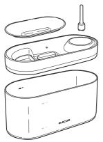
Washing the tray, filter tray, water tank, and pump tube
