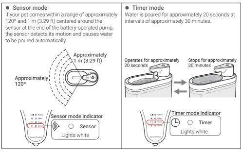
All indicators are off when the product is not operating. To confirm the set mode, press the Power/Mode button. The indicator of the set mode is continuously lit white and water is poured.
