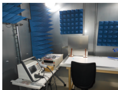
Static electricity testing environment in shielded room
