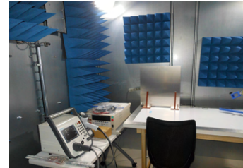
Static electricity testing environment in shielded room
