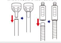
Put the cap and tank on to make it compact so that you can carry it easily.
