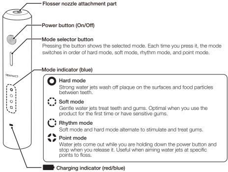
Blinks red when the battery level is low, blinks blue when charging is in progress, and stays lit blue when charging is completed.
