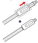
If the parts on both ends of the water hose have come off, push the hose toward the parts to reconnect them.
