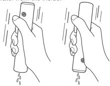
Drain from the water port on the bottom of the main unit and the flosser nozzle attachment part.
