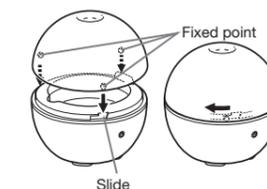
Please make sure whether there is a gap between the main unit and the cover. If yes, the gap may cause water leakage or other faults.
